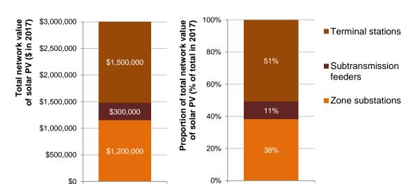
FIGURE 4.2 NETWORK VALUE OF SOLAR PV, BY ASSET TYPE<sup>a</sup> (2017)
