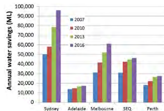
Figure 3: Water savings from rainwater harvesting and water efficient appliances for each region
