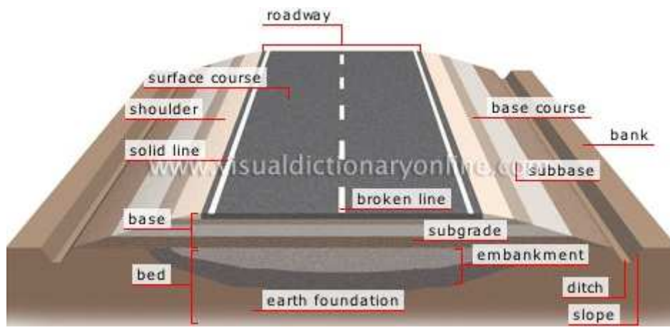
Figure 4 - Typical road cross section
